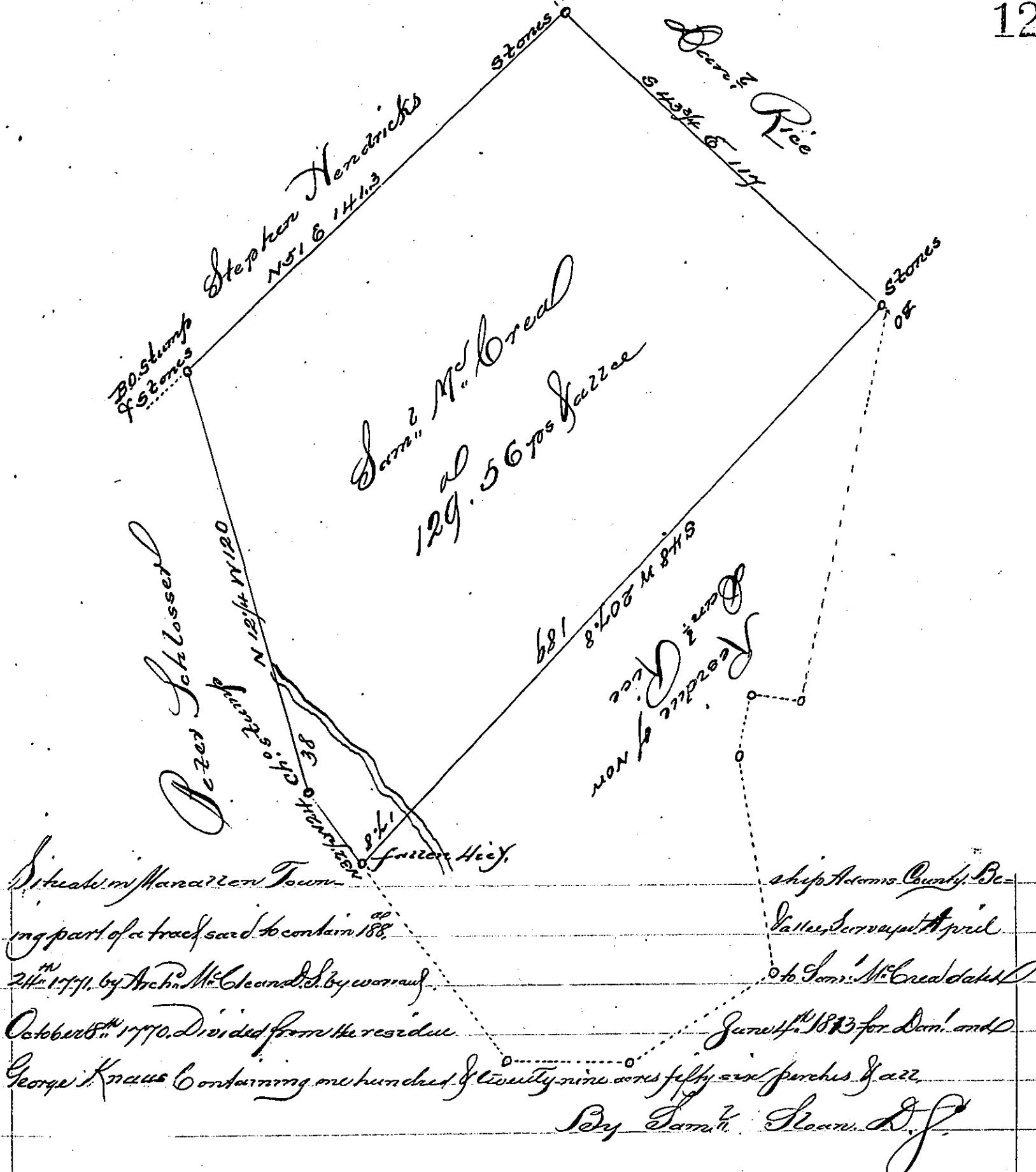
N. B. This survey does not close by 3 perches, nor can it be made to close without doing violent to the courses on the ground owing to mineral attraction. I had all the lines chained twice, the former survey was very erroneous!
